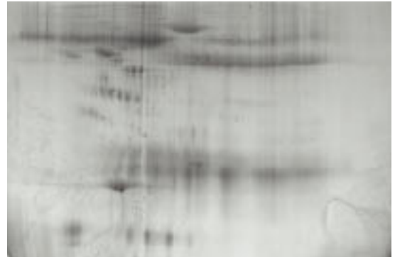
Protein stained with SYPRO® Ruby after 2D electrophoresis (473nm excitation laser with LPG filter)
